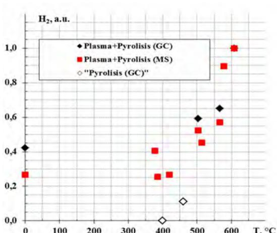
Fig. 1. H<sub>2</sub> intensity (MS) and partial H<sub>2</sub> content in syngas products (GC) after the ethanol reforming vs. Postdischarge pyrolytic chamber temperature
