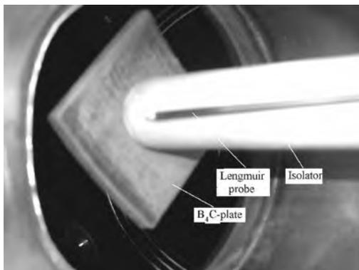
Fig.1. The movable limiter in situ in the branch pipe #1 of the Uragan-2M torsatron
