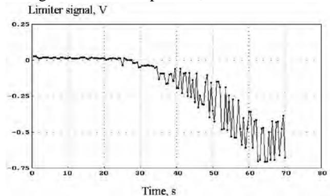
Fig.2. Time dependence of the limiter signal intensity during its moving to plasma axis
