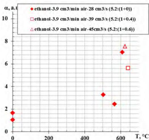
Fig. 2. Energy efficiency of ethanol reforming vs. temperature in the postdischarge pyrolytic chamber
