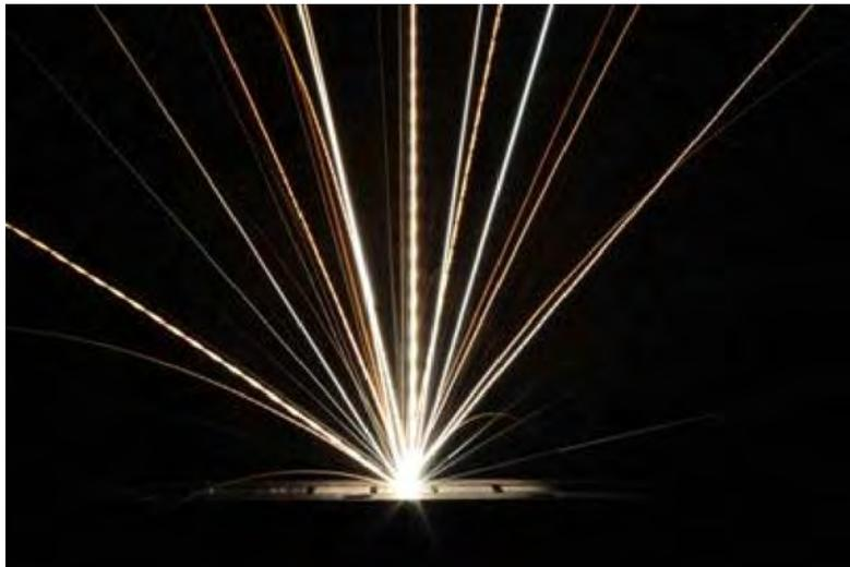
Fig. Brittle destruction of tungsten coatings on CFC substrate during thermal shock in the electron beam facility JUDITH 1 at FZJ (absorbed power density: 237 MW/m<sup>2</sup> for 1 ms)
