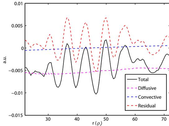
Fig.2. Structure of momentum flux in the CTEM turbulence with  $\omega_\phi = (-0.1 + 0.2 r/a) v_i / R_0$ .
