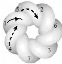
Schematic representation of poloidal-toroidal magnetic surface origination in 7-foil volume
