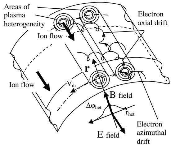
Fig. 1. Electron dispersion on plasma heterogeneities in a stream of ions
