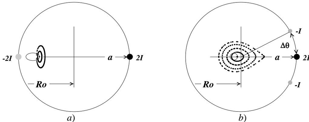
*Poloidal cross-sections of closed magnetic surface configurations and helical coil tracks in a) ordinary  $lm=1$  stellarator and b) modified  $lm=1$  stellarator,  $a/R_o=0.3$*
