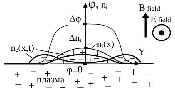
Fig. 2. Distribution of concentration of "motionless" ions  $n_i(x)$  and electrons  $n_e(x,t)$  changing in phase in the field of plasma heterogeneities
