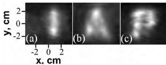
bremsstrahlung continuum from the PC increases in the visible region when the plasma electrons are heated by millimeter waves. As an example, the near-field MMW images of the slits in the foils that have shapes of the letters I, A, and P from acronyms for Institute of Applied Physics obtained using the technique are shown in Figure [2].
