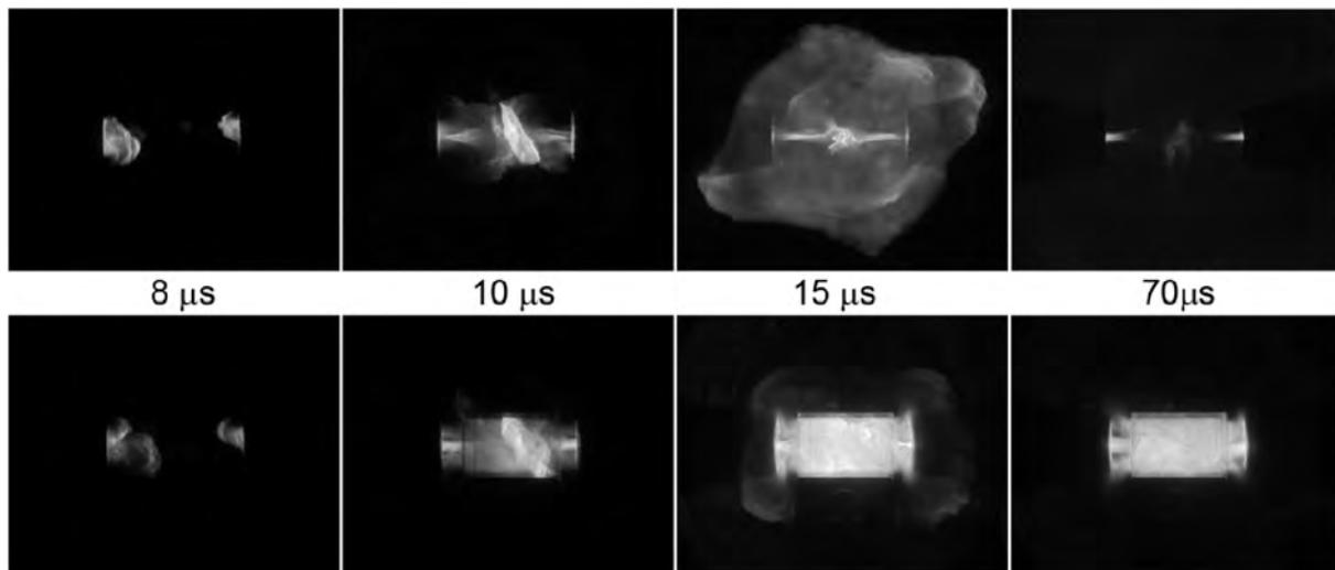
Collision dynamics of erosion plasma counter-flows in the unconfined area (top) and in the area confined by a quartz tube (bottom)
