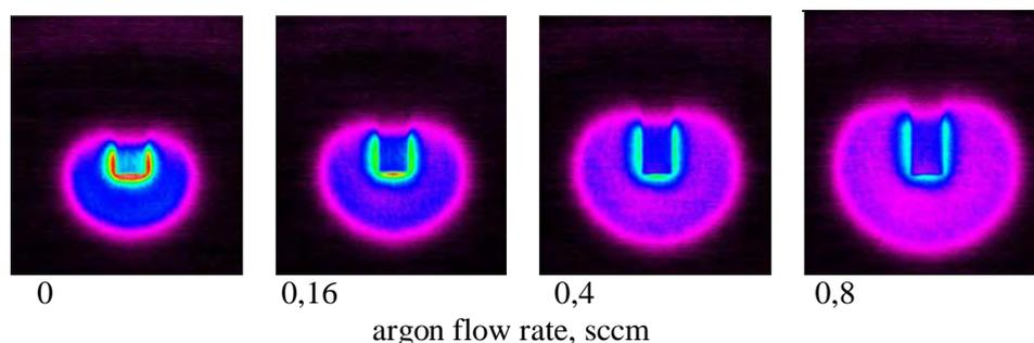
Influence of the Ar content on the N<sub>2</sub> EMD image (N<sub>2</sub> flow rate 10 sccm).
