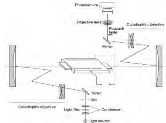
Fig.2 Experimental setup for optical measurements
