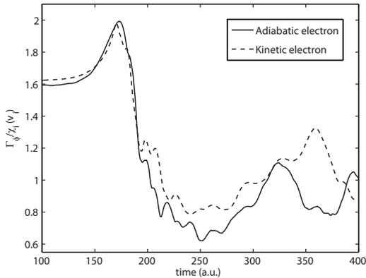
Fig.1. Time evolution of the ratio of the momentum to heat flux in the ITG turbulence with adiabatic (solid) and with kinetic electrons (dashed line).
