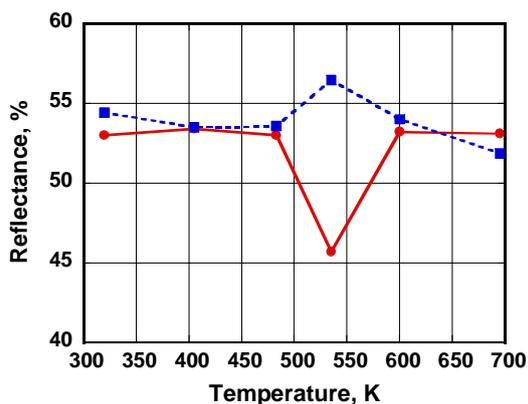
Fig. 1. Reflectance of specimens ( $\lambda=632.8$  nm) exposed at different temperatures
