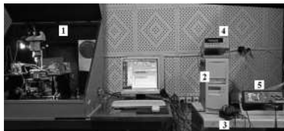
Fig. 2. A computerized stand for measuring the statistical characteristics of planar detectors: 1 - manual test station; 2 - computer; 3 - switching unit; 4 - picoammeter KEITHLEY model 6487; 5 - RLC meter - BK Precision 8953
