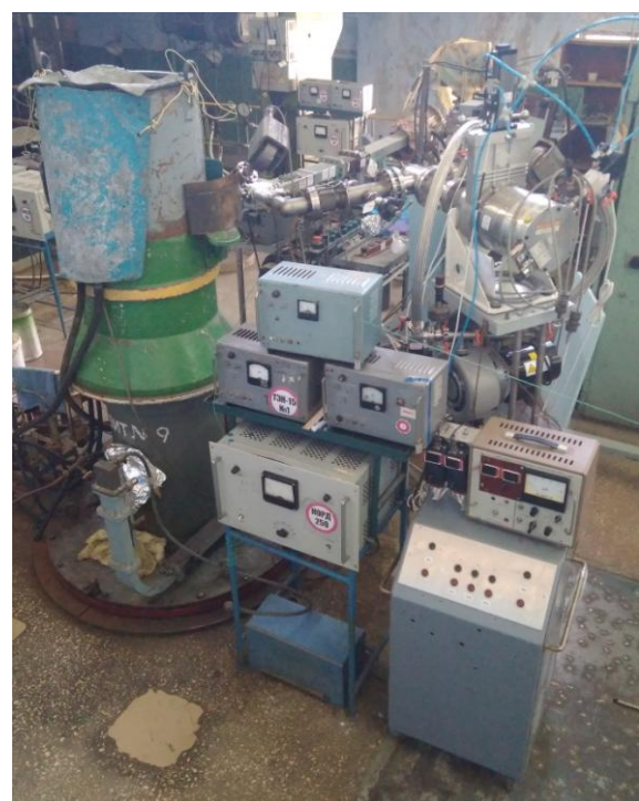
Fig. 6. Configuration of vacuum system during HV and RF training of klystron
