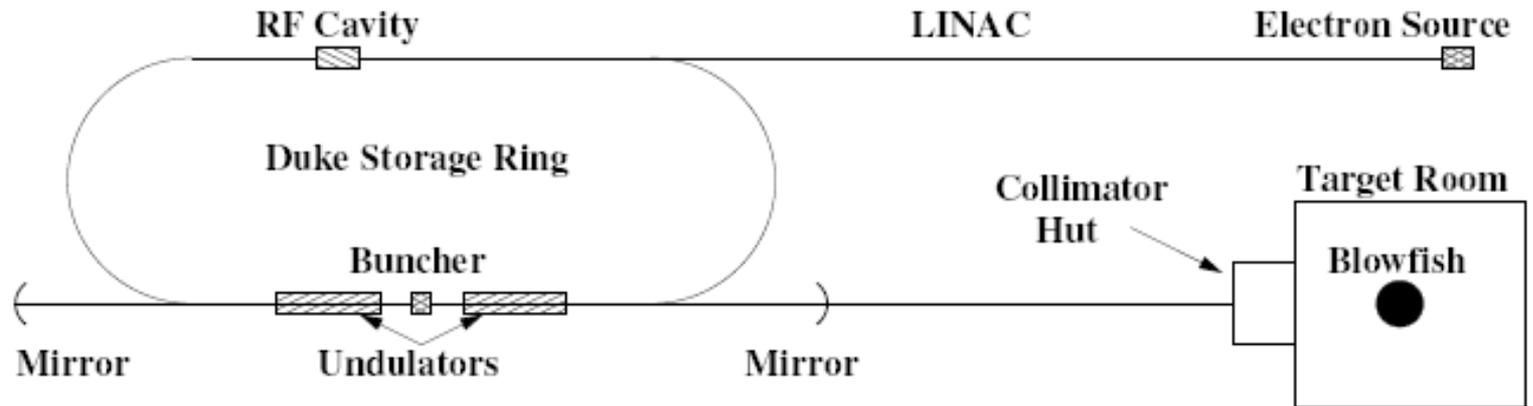
The wide-acceptance neutrons detector: **Blowfish Detector Array**.
