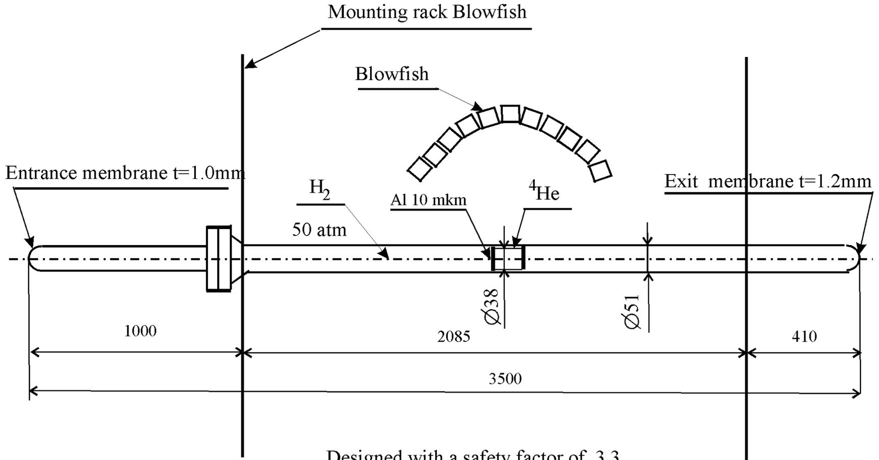
A gas target provides possibility of turn of Blowfish on a angle  $\varphi = 90^\circ$
