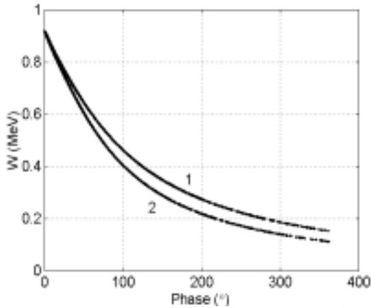
Fig. 3. Phase-energy electron distribution at the single-cavity RF gun output. 1 – thermoemission, 2 - photoemission.
