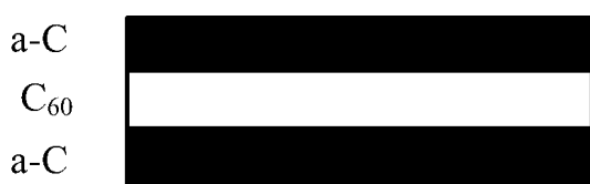
Fig. 2. “Sandwich” structure a-C/ C_{60} /a-C.
