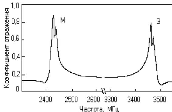
Fig. 2. The graph of the dependence of the reflection factor on the frequency of the dielectric sphere from  $\text{TiO}_2$ , with 13.20 mm in diameter placed in the center of the rectangular waveguide.
