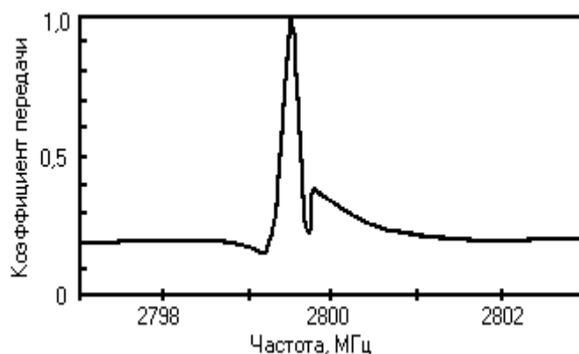
Fig. 3. Transfer ratio versus the frequency of a single dielectric disc from  $TiO_2$  of the thickness of 3.291 mm, with the central hole of 5 mm in diameter in a circular half endless waveguide of 81.5 mm in inner diameter  $E_{01}$  oscillations have been excited.
