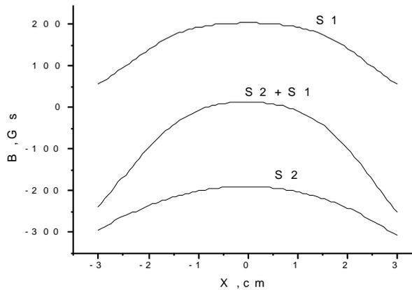
Fig. 4. Making sextupole component in a quadrupole lens.
