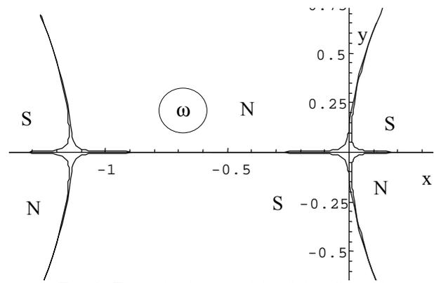
Fig. 1. The pole shapes of the "ideal" quadrupole+sextupole lens. Measurements are in meters.  $G_2=20T/m$ ,  $G_3=35T/m^2$ .
