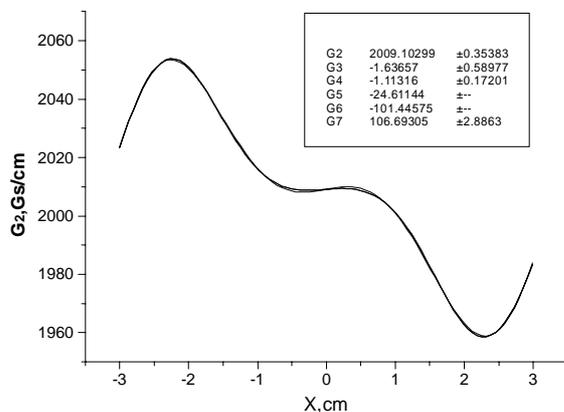
Fig. 5. Distribution of the gradient in lens in a mode of compensated sextupole component.
