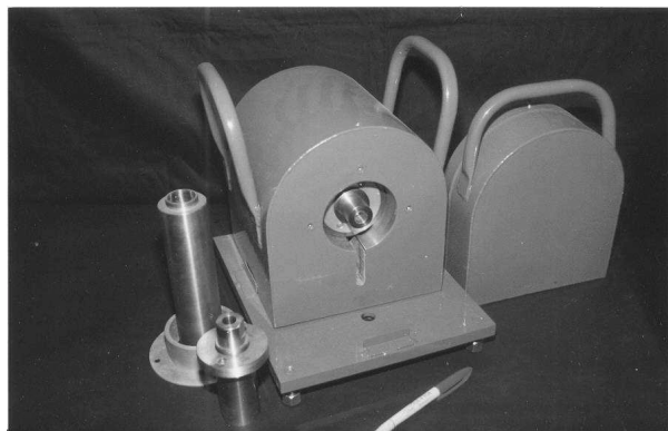
Fig. 2. Co-57 source into shield block with a set of collimators.
