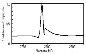
Fig. 3. Transfer ratio versus the frequency of a single dielectric disc from  $TiO_2$  of the thickness of 3.291 mm, with the central hole of 5 mm in diameter in a circular half endless waveguide of 81.5 mm in inner diameter  $E_{01}$  oscillations have been excited.
