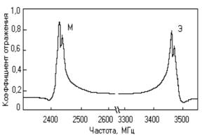
Fig. 2. The graph of the dependence of the reflection factor on the frequency of the dielectric sphere from TiO<sub>2</sub>, with 13.20 mm in diameter placed in the center of the rectangular waveguide.
