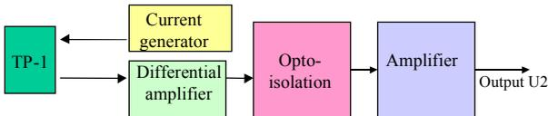
Fig. 6. Block-diagram of temperature measurement circuit.
