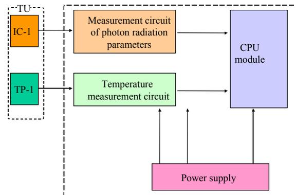
Fig. 4. Block-diagram of measurement channel.
