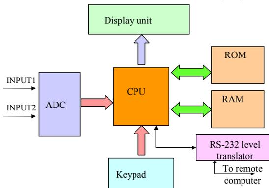
Fig. 7. Block-diagram of the CPU module.
